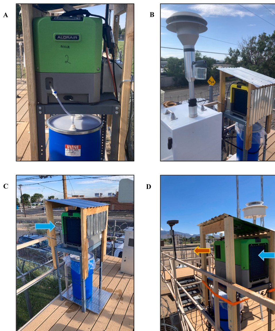
Fig. 2. (A) AWH unit at the urban site with the outlet for the water collection into the 15-gallon lined drum. (B) MetOne E-SEQ FRM for particulate matter monitoring. (C) AWH unit at the urban site. From the bottom up, Arlyn scale with 15-Gallon water collection bin sitting on top, with tubing connecting the dehumidifier to the bin. (D) Blue arrow shows air input through a large side panel into the dehumidifier, orange arrow shows dry air output.
